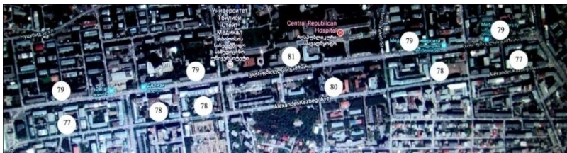
Fig. 2. The map of Vazha Pshavela and Alexander Kazbegi avenues (one-way traffic) with indicated maximum values of L_{Aeqv} (dBA).
